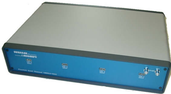
Fig. 1: Customer specific layout of Fourfold Quad Channel USB2.0-TDC operating in R mode with 16 stop channels on 4 HDMI connectors.
